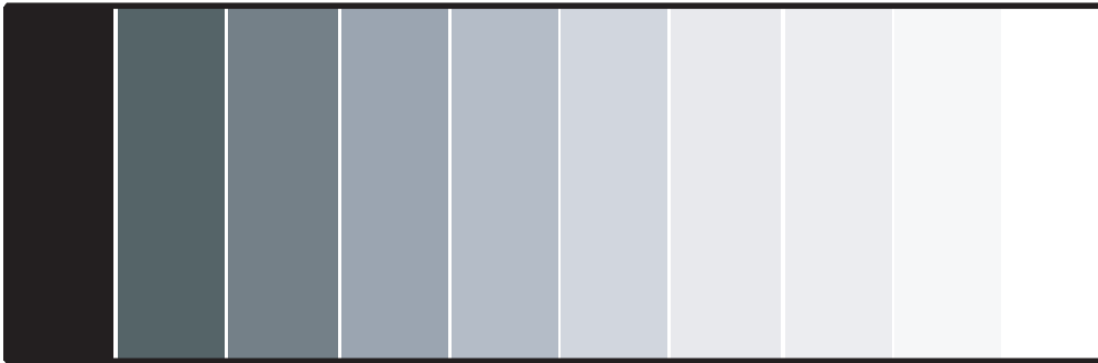
Figure 4-3. Typical Gray Bar Pattern for Adjusting Contrast
